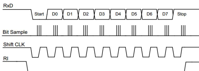
Figure 13-12 Receive Timing of Mode 1
