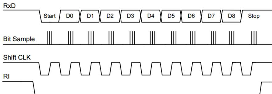
Figure 13-14 Receive Timing of Mode 2
