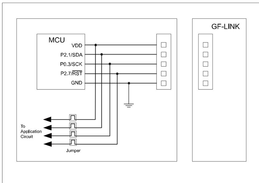
Figure 3-1 GF-LINK 编程硬件连接
